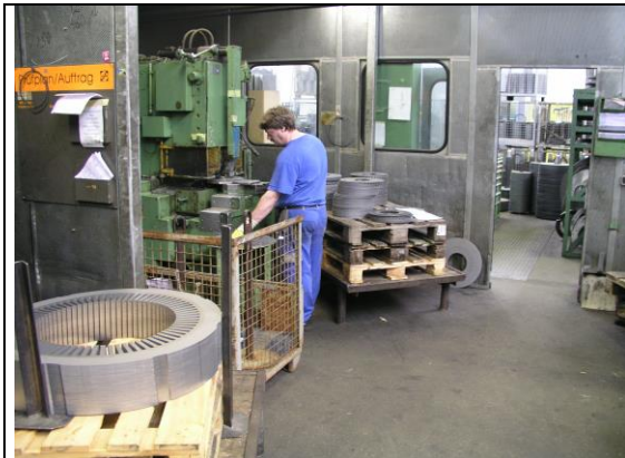
Abb. 8.5: Nutenstanze in Kabine
