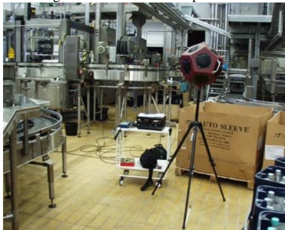
Figure 2 – Dodecahedron loudspeaker in a production hall
