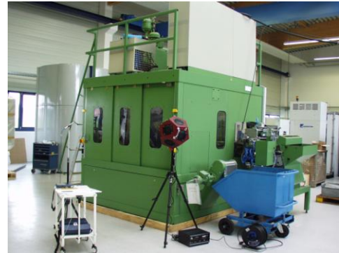
Figure 6: Encapsulated machine with three emission areas
