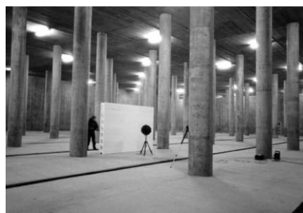
Figure 18: Measuring the screening effect with a transportable screen in a retention basin
