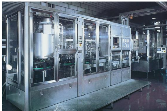
Figure 4: Filling machine in a bottling plant
