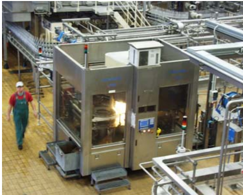
Figure 6: Enclosure of a machine with open deck.
