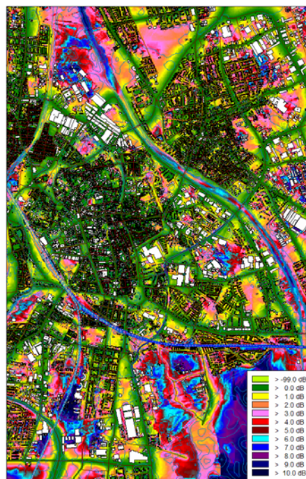
Figure 5: Level differences in a city (80000 buildings) between a calculation with favorable conditions and one with homogenous conditions according to NMPB [2]
